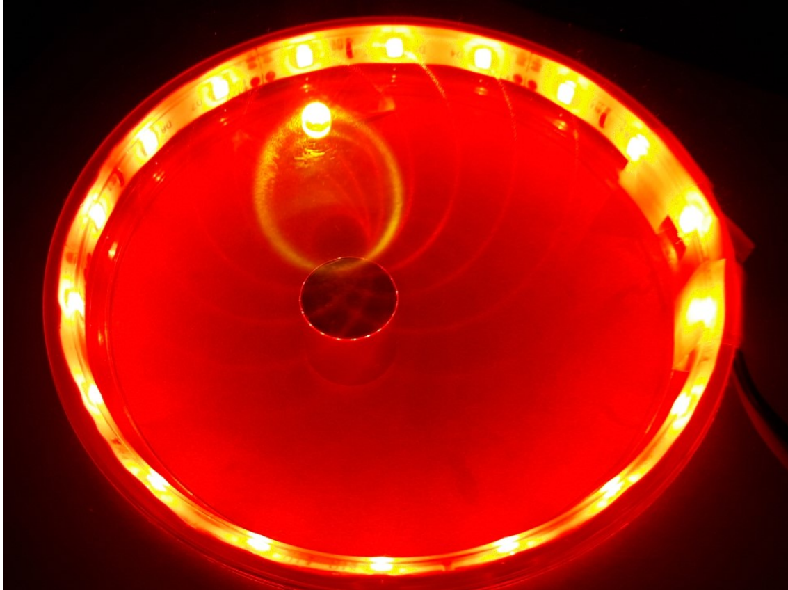
Figure 2.7 - View in perspective of a setup with a circular frame of red LEDs, with a white LED within this frame.
