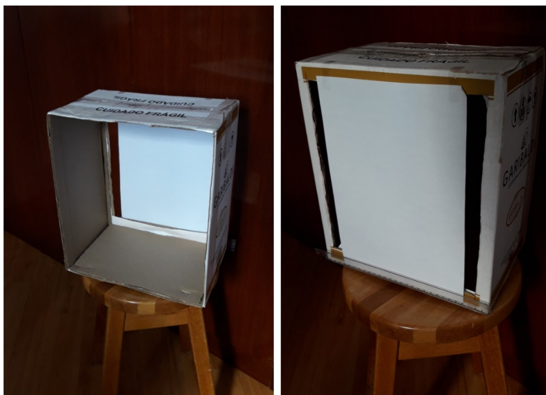
Figure 3.11 - Two views of a white sheet paper supported in a cardboard box. Hanging a ruler at the bottom of the sheet helps to keep the paper well stretched to prevent deformation of the images.
